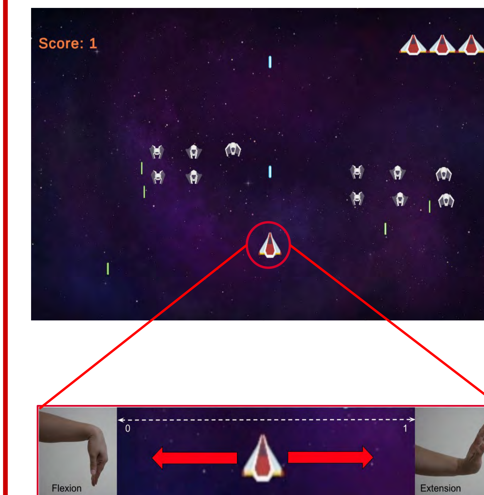
Figure 7. Video game interface. The game requires horizontal movement to shoot enemies. We utilized an extensor ratio (shown below), so that independent activation of the ECR through extension would move the ship to the right and independent activation of FCR would move the ship to the left.
