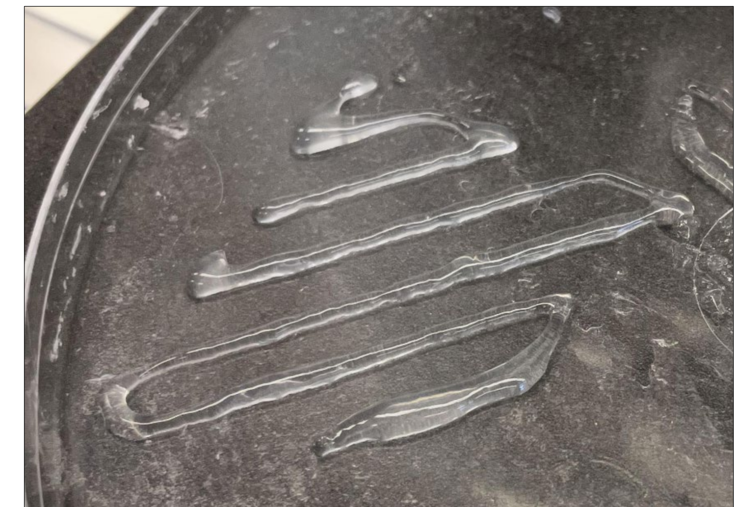
Figure 4: First layer of scaffold printed with dimensions of 30mm x 30mm using 5% gelatin hydrogel, 18 gauge needle, and feed rate of 85 mm/min. There are definite uniform lines, and no blobbing.
