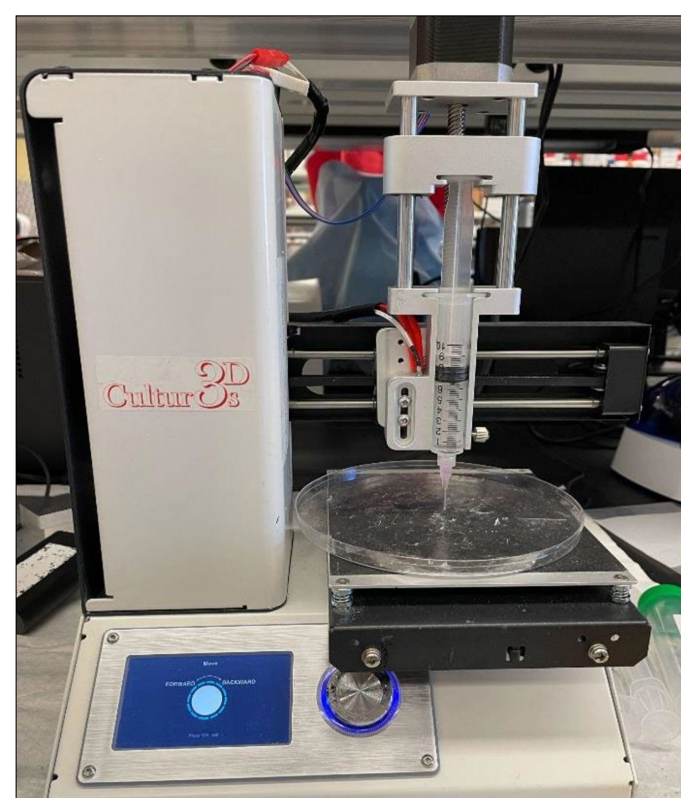
Figure 2 (left): 3D Cultures TissueScribe Printer. 10 mL syringe with 18 gauge needle is inserted into printer loaded with 5% gelatin hydrogel solution.
